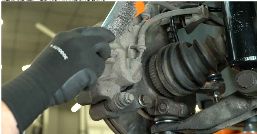
10 Unscrew the lower brake caliper fastener. Use an 13 mm socket. Use a ratchet wrench.
