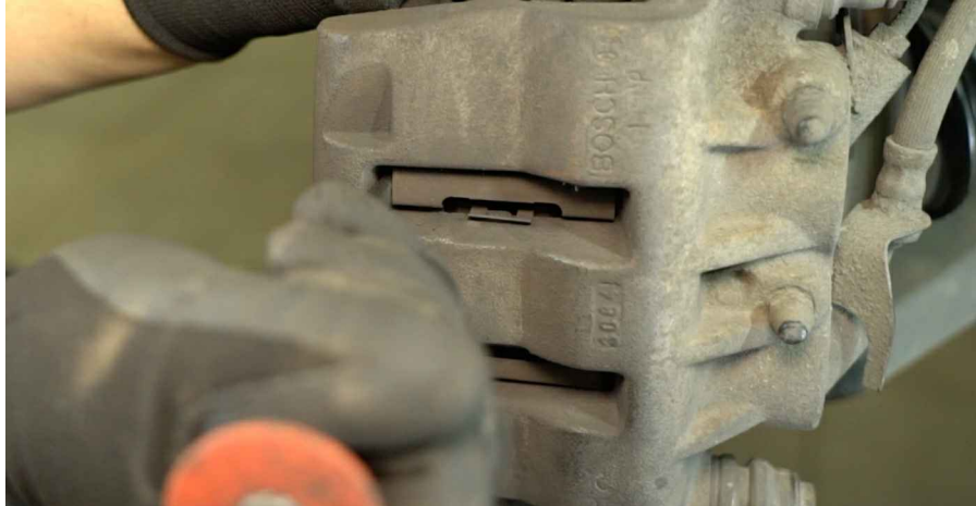
9 Clean the brake caliper fasteners. Use a wire brush. Use WD-40 spray.
