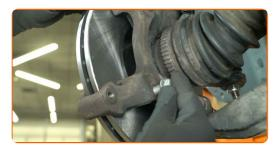
Tighten the fasteners of the brake caliper bracket. Use an 18 mm socket. Use a torque wrench. Tightening torque: 110 N·m.
