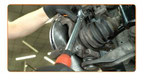
Remove the brake pad anti-rattle clip from the brake caliper.
