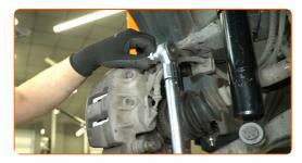
Tighten the lower brake caliper fastener. Use an 13 mm socket. Use a torque wrench. Tightening torque: 30 N·m.
