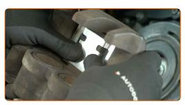
Treat the brake pads in the areas where they contact the brake caliper bracket. Use anti-squeal paste.
