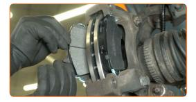
38 Install the brake caliper.
