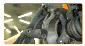
Clean the brake disc screw. Use a wire brush. Use WD-40 spray.
