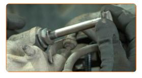
13 Remove the brake caliper.
