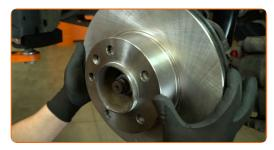
26 Install the brake disc screw.
