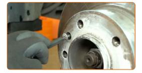
Remove the brake disc.
