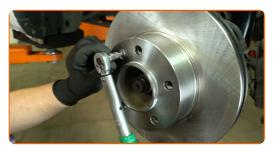
Clean the brake caliper bracket and check its condition. Use a wire brush. Use a brake cleaner.
