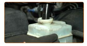
Tighten the brake fluid reservoir cap.
