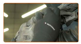
Tighten the upper brake caliper fastener. Use an 17 mm socket. Use a torque wrench. Tightening torque: 80 N·m.
