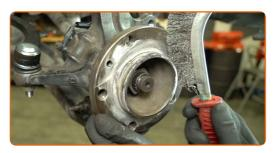
Treat the wheel hub surface that is in contact with the brake disc. Use ceramic grease.
