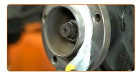
25 Install a new brake disc.
