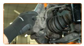
Unscrew the lower brake caliper fastener. Use an 13 mm socket. Use a ratchet wrench.
