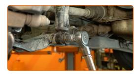
Tighten the fastener that connects the control arm to the subframe. Use a 30 mm socket. Use a torque wrench. Tightening torque: 280 N·m.
