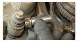
Unscrew the pinch bolt that connects the lower ball joint to the steering knuckle. Use a 16 mm combination spanner. Use an E16 Torx socket. Use a ratchet wrench.
