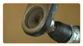
Install a new ball joint. Use a ball joint C-frame press kit.
