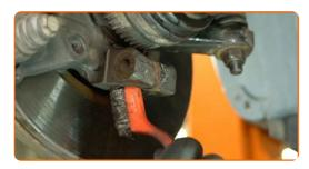
Remove the retaining ring from the ball joint boot. Use a slotted screwdriver.
