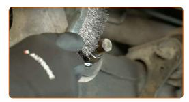
Loosen the fastener that connects the control arm to the subframe. Use a 30 mm socket. Use a tommy bar.
