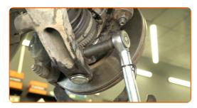
Install the lower fastening bolt of the brake caliper bracket.
