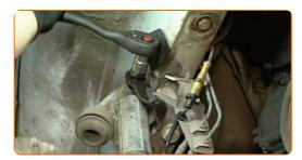
Unscrew the lower fastener of the shock absorber. Use a 21 mm socket. Use a ratchet wrench.
