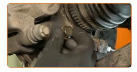
Tighten the lower fastener of the brake caliper bracket. Use an 18 mm socket. Use a torque wrench. Tightening torque: 110 N·m.
