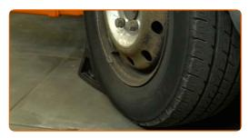
Loosen the wheel fasteners. Use a 24 mm wheel impact socket. Use a tommy bar.
