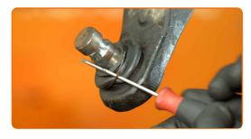
Remove the ball joint boot. Use a slotted screwdriver.
