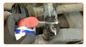
Unscrew the upper fastener of the shock absorber. Use an 18 mm socket. Use a ratchet wrench.
