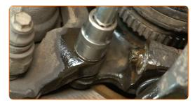
17 Remove the fastening bolt.
