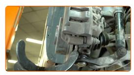
Clean the fastener connecting the control arm to the subframe. Use a wire brush. Use WD-40 spray.
