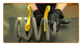
Install the spring compressor on the new spring.
