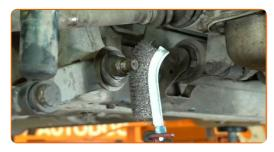
Loosen the fastener connecting the control arm to the subframe. Use a 30 mm socket. Use a tommy bar.
