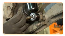
To tighten the fasteners correctly, you have to jack up the suspension to load it. Use a transmission jack or one more vehicle jack.
