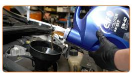
Replacement: engine oil and filter – NISSAN INTERSTAR Box (X70). Tip from AUTODOC:
