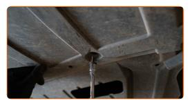
Remove the oil pan cover. Use a drive socket #10. Use a flat screwdriver.
