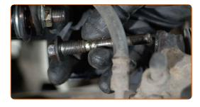
10 Remove the brake caliper.
