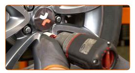
Lower the car and working in a cross order, tighten the wheel bolts. Use wheel impact socket #21. Use a torque wrench. Tighten it to 118 Nm torque.
