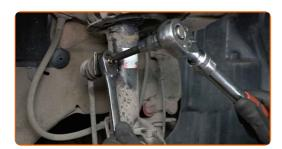
Unscrew the fastener connecting the stabilizer link to the stabilizer bar. Use a combination spanner #17. Use HEX No.H5. Use a ratchet wrench.
