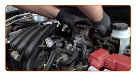
Tighten the throttle valve fasteners. Use a drive socket #8. Use a torque wrench. Tighten it to 10 nm torque.
