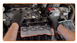
27 Install the intake manifold.
