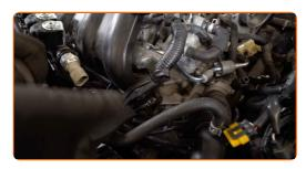
11 Remove the intake manifold.
