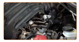
Cover the intake manifold passages with a microfibre towel to prevent dust and dirt from getting inside.
