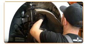
Unscrew the fuel filter bracket fixing bolts. Use a drive socket #13. Use a ratchet wrench.
