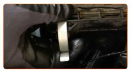
4 Slightly raise the cover of the air filter housing.
