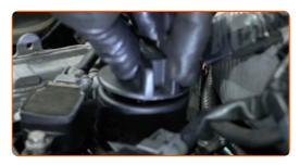
Tighten the oil filler cap.
