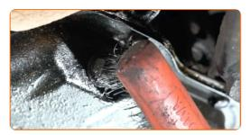
8 Unscrew the drain plug. Use a drive socket #14. Use a ratchet wrench.
