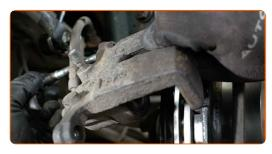
Install the brake caliper guide pins.
