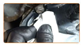
Screw in the new drainage plug and tighten it. Use a drive socket #14. Use a torque wrench. Tighten it to 30 Nm torque.
