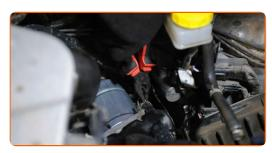
Tighten the fastening clamps of the fuel filter pipes. Use pliers.
