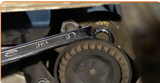
**49** Remove the serpentine belt tensioner pulley.
