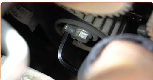
**43** Pull aside the timing belt tensioner pulley.
