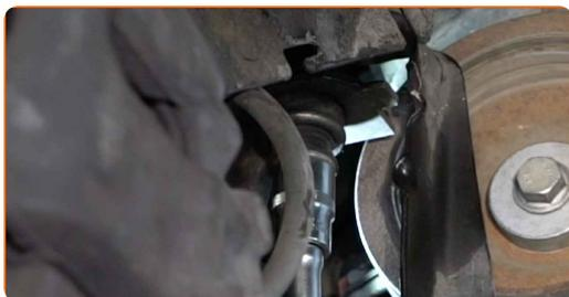
**99** Install the fuel filter fastening bracket.
