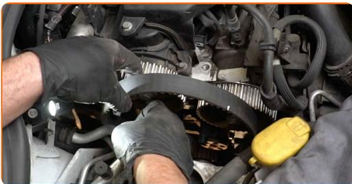
**45** Return the tensioner pulley to its initial position.
