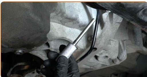
**92** Screw in the TDC timing pin plug. Use a drive socket #E14. Use a ratchet wrench.
