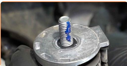
**85** Install the serpentine belt tensioner pulley.
