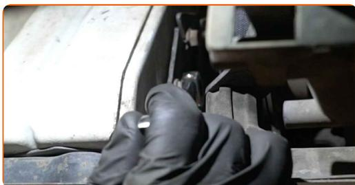
**101** Install the fuel filter fastening bracket.
