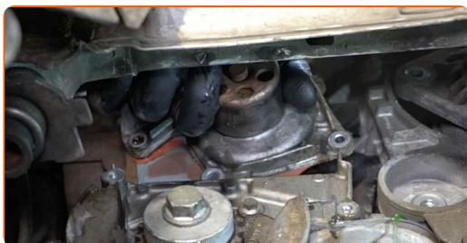
Replacement: water pump & timing belt kit – NISSAN ALMERA II Hatchback (N16). Tip:
