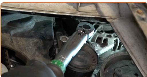
**87** Unscrew the crankshaft pulley fastener. Use a drive socket #18. Use a ratchet wrench.
