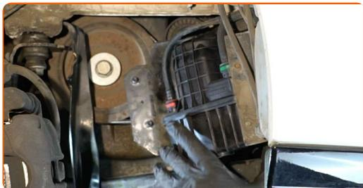
**100** Screw the fixing bolts of the fuel filter bracket. Use a combination spanner #10.
