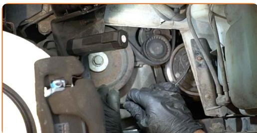
**18** Return the tensioner pulley to its initial position. Use a combination spanner #16.
