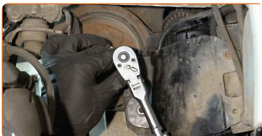
**103** Install the wheel arch cover to its mounting seat.
