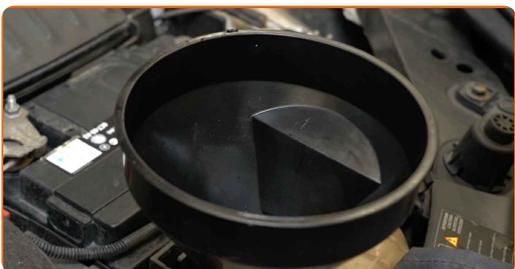
**112** Pour coolant in the coolant reservoir.
