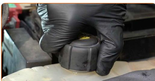
**119** Check the coolant level. If necessary, top up to the required level.
