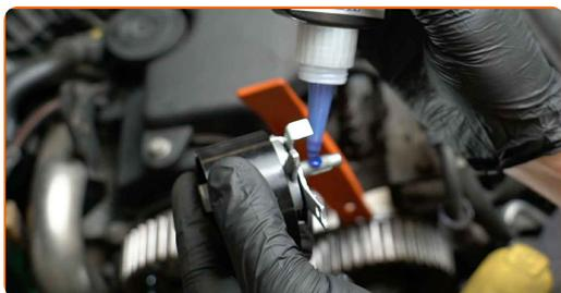
**67** Install the timing belt tensioner pulley.
