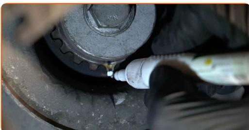
**42** Loosen the fastener of the timing belt tensioner pulley. Use a combination spanner #13. Use HEX No.H6.
