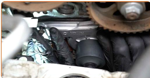
**63** Tighten the water pump fasteners. Use a drive socket #8. Use a torque wrench. Tighten it to 12 Nm torque.
