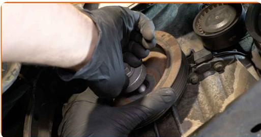
**89** Install the crankshaft pulley locking tool. Use an engine timing tool set.
