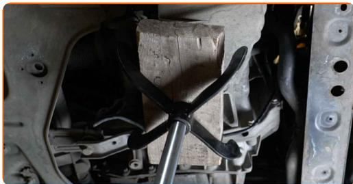
**32** Unscrew the upper fastener of the engine mount. Use a drive socket #16. Use a ratchet wrench.
