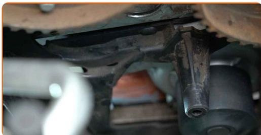
**65** Screw in the fasteners of the middle timing cover. Use a drive socket #8. Use a ratchet wrench.
