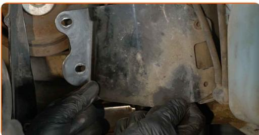
**14** Unscrew the fuel filter bracket fixing bolts. Use a combination spanner #10.
