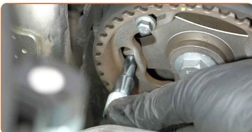
**41** Make a mark on the camshaft gear.
