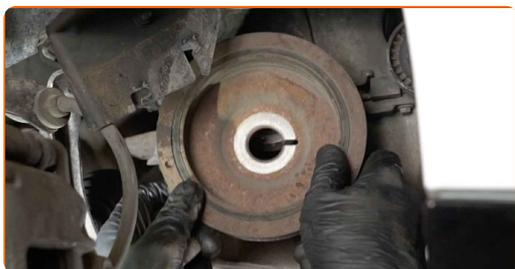
**28** Screw in the crankshaft pulley fastener. Use a drive socket #18. Use a ratchet wrench.
