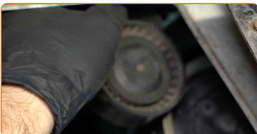
**86** Tighten the fastener of the serpentine belt tensioner pulley. Use a drive socket #13. Use a torque wrench. Tighten it to 35 Nm torque.
