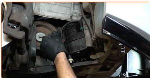
**16** Pull aside the V-ribbed belt tensioner pulley. Use a combination spanner #16.
