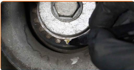
**40** Install the camshaft gear locking tool according to the factory marks. Use an engine timing tool set.
