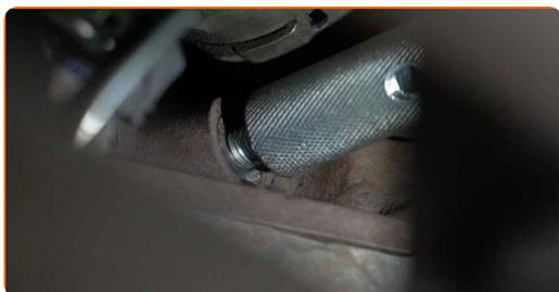
**26** Unscrew the crankshaft pulley fastener. Use a drive socket #18. Use a ratchet wrench.
