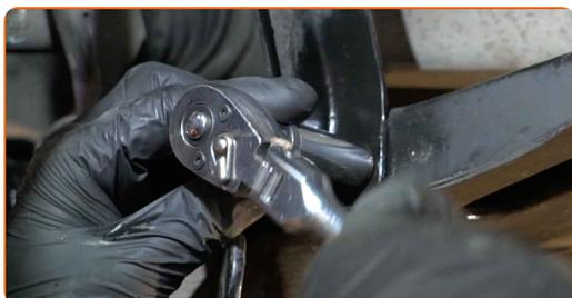
**22** Unscrew the subframe fastening. Use a drive socket #18. Use a ratchet wrench.
