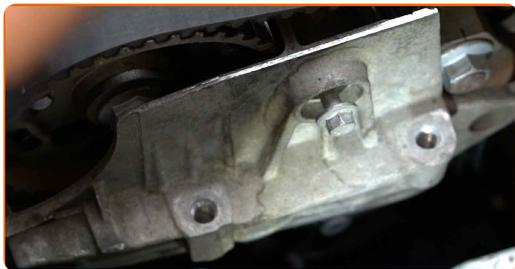
**77** Tighten the engine mount fastening bolts. Use a drive socket #10. Use a torque wrench. Tighten it to 40 Nm torque.
