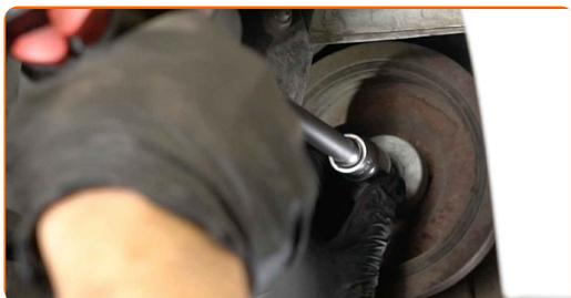
**27** Remove the crankshaft pulley.
