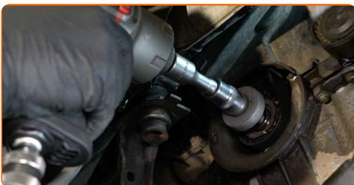
**88** Install the crankshaft pulley according to the factory marks.
