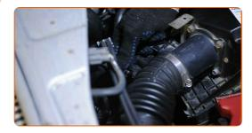
Connect the crankcase ventilation hose to the air duct.
