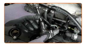
6 Clean dirt, dust and debris from inside the spark plug wells.
