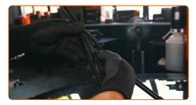
Remove the blade from the connector
