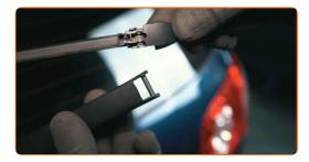
19 Install the new wiper blade and fasten it
