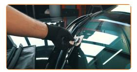
Alternatively, you can use one hand to hold the arm and the other hand to mount the new blade
