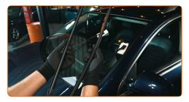
Replace the arms if they've corroded or fail to press the blades against the windscreen sufficiently
