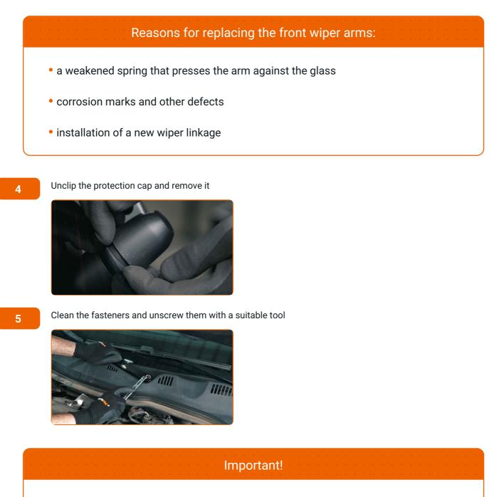
• Hold the arm firmly to avoid damaging the pivot shaft
