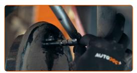
Check that the threaded part of the brake pipe fitting is in line with the thread in the mounting hole
