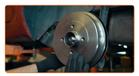
Press the brake pedal and engage and release the parking brake lever several times. This will centre the brake shoes in relation to the circumference of the drum
