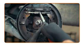
Clean the working area on the back of the backing plate
