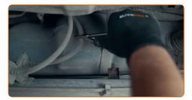
To prevent the brake pipe from turning, loosen the connection by rotating it gradually
