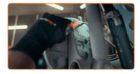
When unscrewing the pipe, clamp off the nearest flexible connection to avoid a brake fluid leak
