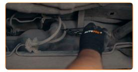
The system is bled by pumping the brake pedal Repeat the procedure until there are no air bubbles left in the fluid
