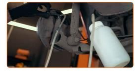
Remove the clamp from the flexible brake hose
