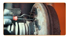
If there is no adjuster access hole, the procedure can be carried out via the wheel bolt hole
