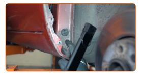
Insert the wheel arch liner into the mounting seat
