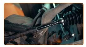
Loosen the additional fastener and unscrew the tie rod end from the tie rod
