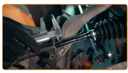
Maintain this value when installing a new tie rod end
