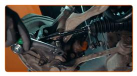
Treat the fasteners with an anti-corrosion agent
