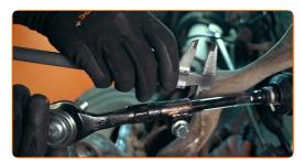
After installation, check that the length of the threaded portion is the same as before
