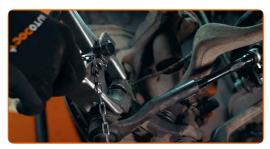
The connection between the tie rod end and the tie rod is adjustable
