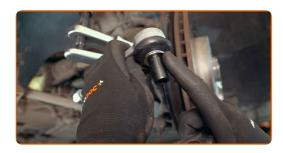
Unscrew the tie rod end while holding the tie rod
