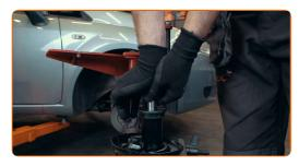
When reassembling the strut, be sure to use new seals
