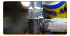
Use a wire brush on the mounting seat. Use a grinder if necessary.
