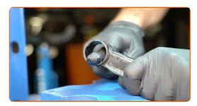
Press the new bush in. Make sure that the bush is inserted at a 90-degree angle. Otherwise, you can damage both the bush and the component it is installed in.
