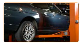
2 Unscrew the wheel fasteners and remove the wheel.
