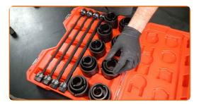
Identify the bush type: rubber or with a metal or plastic shell. Depending on the bush type, you may need a pulling spindle in addition to a press or vice.
