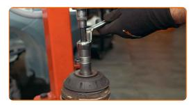
Replace the component and carefully inspect the bump stop, the dust boot, the spring, and the strut itself
