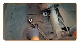
The suspension strut can be either bolted to the steering knuckle, fitted into the mounting seat on the knuckle, or attached to the suspension arm
