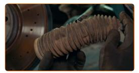
Clean the steering rack shaft of old grease and dirt and apply some new grease
