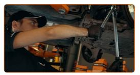
Treat the fasteners with an anti-corrosion agent
