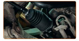
Screw on the lock nut, using your mark as reference
