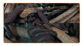
Remove the lock nut carefully so as not to erase the mark
