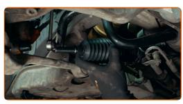
Make sure the boot fits tightly to its mounting seats and is secured reliably
