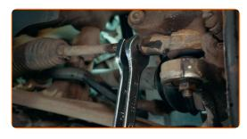
Unscrew the tie rod end from the tie rod
