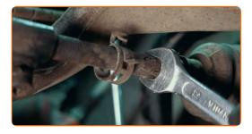
Remove the dust boot fasteners and take the boot out
