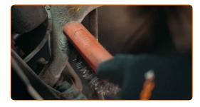
Measure the distance from the beginning of the threaded portion on the tie rod to the tie rod end, not to the lock nut
