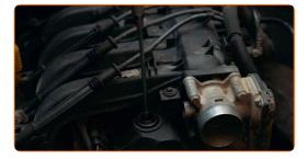
Select a spark plug socket of the required size and lower it into the spark plug well
