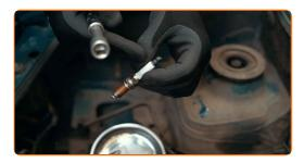
Secure the component in the spark plug socket and lower it carefully into the spark plug well
