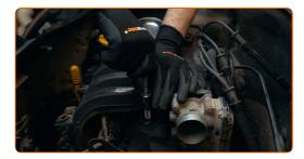
Tighten them with a torque wrench to the manufacturer's recommended torque
