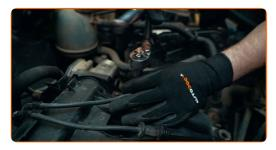
Remove the spark plugs from their wells. A special magnetic socket can be used for this
