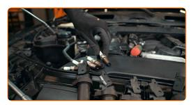
Apply high-temperature grease to the thread of new plugs and dielectric grease to the insulator
