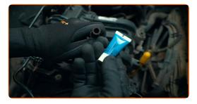
Prevent dielectric grease getting on the electrodes to avoid ignition system malfunctions
