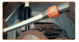
Replacement of the dust boot and bump stop on a suspension strut
