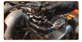
Remove the hoses from the reservoir and drain out the rest of the old fluid from the return hose into the prepared drain pan.
