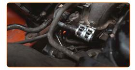
Pour in the new power steering fluid. The type and amount to use is specified by the car manufacturer.
