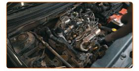
If the oil filter is installed on the underside of the engine, you'll need to remove the engine splash guard
