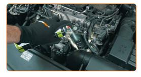
Unscrew the oil filter cap or the filter itself
