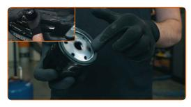
25 If the filter is a cartridge style one, remove it from its mounting seat on the cap
