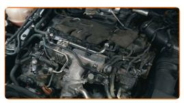
The oil filler. This is located on the top of the engine
