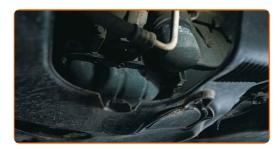
The drain plug. It is located under the engine in its oil pan
