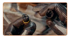
Using a special socket and ratchet wrench, unscrew the lambda sensor by rotating it counterclockwise.
