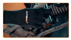
Unscrew the tie rod, having first secured the tie rod end
