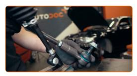
Before installing the new component, clean the steering rack shaft of old lubricant and apply some new
