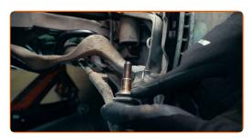
To access the fastener on the steering rack shaft, remove the boot clamps and the boot
