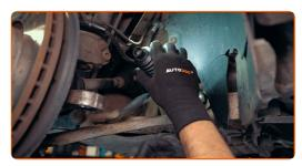
or make a mark on the threaded portion of the tie rod, mount it on the rack, and put the boot on
