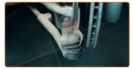
Clean the fastener that connects the part to the steering knuckle
