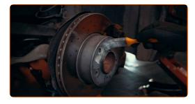
Clean the working surface of the brake disc
