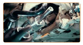
Apply some threadlocker to the threaded portion and screw in the new tie rod
