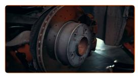
Treat the surface with an anti-corrosion agent
