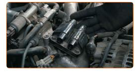
If there is a lock on the electrical connector, unclip it
