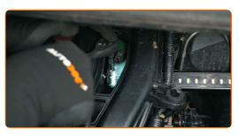
Remove the ignition coil from its mounting seat
