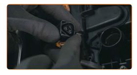
Install the new ignition coil in the mounting seat
