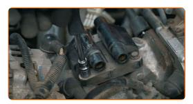
Check the high voltage wires for damage and corrosion of the connectors
