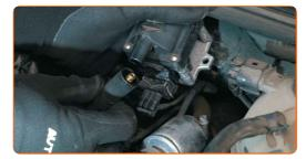
Draw the wires to different sides to prevent mixing them up when reinstalling
