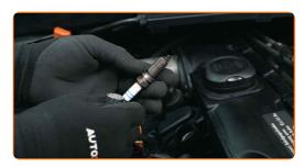
Check that there are no signs of corrosion on the connectors, and that the seals and the wiring harness are in good condition
