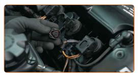
22 If the electrical connector has a lock, release it
