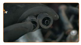
14 Install a new ignition coil in the mounting seat
