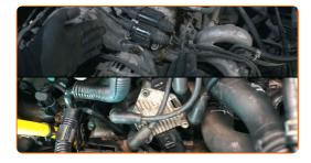
6 Pry up and unclip the caps of the high voltage cables
