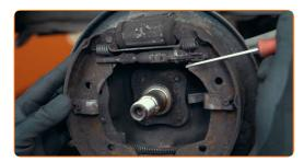
First, remove the parts securing the brake shoes. Use a fork-type screwdriver or a special toolkit
