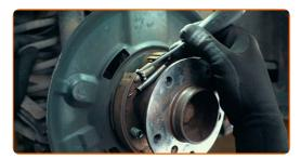
The adjuster gear can be accessed via the wheel bolt hole or the hole in the hub
