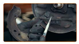
Disconnect the cables from the handbrake control lever
