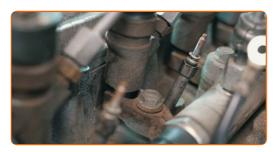
If the glow plugs are difficult to access, use a magnetic pickup tool with a flexible shaft
