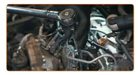
Set the wrench to the torque value recommended by the car manufacturer. This value may be specified on the package or in the car repair manual
