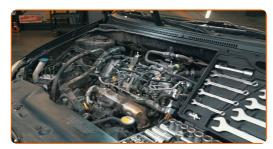
Open the bonnet and remove the engine cover
