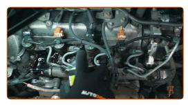
To unscrew the glow plugs, use a torque wrench with a suitable socket
