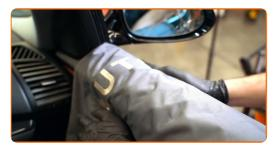
2 Protect the paintwork of the mirror housing. Use the masking tape.
