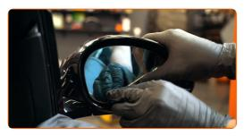
Check if the mirror glass has retaining clips.
