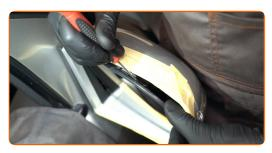
Carefully release the mirror glass from its attachment.
