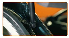
Press the gas strut onto the ball attachment
