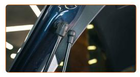
The fitting includes a metal clip. Pry it up using a flathead screwdriver
