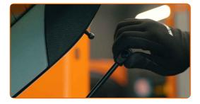
Check whether the gas struts are functioning properly
