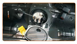
Fuel filter hoses are usually fastened with quick connectors
