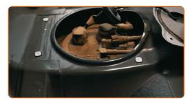
If the fuel filter is located in the tank, a cover is provided under the rear seat or in the luggage compartment floor for easy access to it
