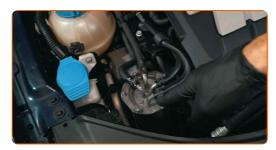
Carefully pry off the fuel filter cover using a suitable tool
