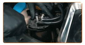
Remove the cover and extract the filter element
