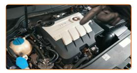
Unscrew all fasteners of the fuel filter cover
