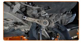
Clean the mounting seats and prepare new fasteners
