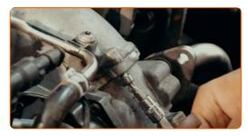
Using a cloth and the cleaner, remove dirt from the valve mounting seat.
