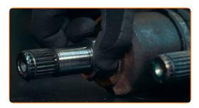
When installing the new CV axle, turn it slightly so that it fits into the splined mating part
