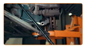
The outer CV joint splines usually get stuck to the hub, so it should be knocked out
