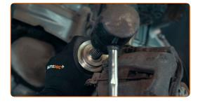
Clean all the mounting seats and secure the outer part of the CV axle
