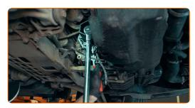
If the CV axle is inserted in the differential, drain the transmission fluid first
