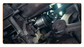
Make the CV axle snap into place by hitting the back end of it with a mallet
