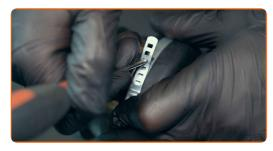
Alternatively, you can use side or end cutting pliers to tighten the clamp and then use a hammer to tap the spot where it was tightened
