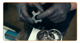
Apply most of the grease to the inside of the CV joint while working the joint by hand at the same time
