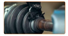
To replace the inner CV boot, remove the larger clamp
