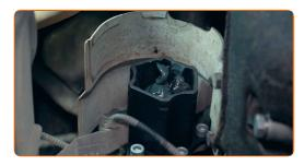
Install the CV axle together with the joint and work the joint by hand to distribute the grease evenly
