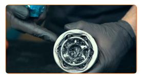
Slide the boot farther away from its mounting seat on the axle shaft so that it does not get in the way while you are working.
