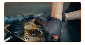
Put a new boot on the axle shaft
