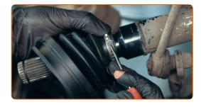
27 Install the thrust washer and plastic bushing
