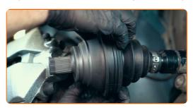
Make sure that the clamps are installed correctly and that the boot is fitted in its mounting seat
