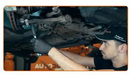
Use a torque wrench to tighten the axle fastener.
