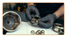
Use special grease for CV joints
