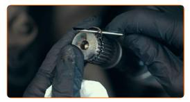
Remove the boot and clean the old grease off the CV joint
