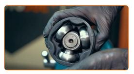
Pack the CV joint housing with the required amount of grease
