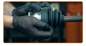
Make sure that the boot does not turn and fits snugly around the CV joint housing
