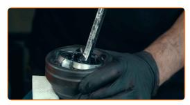
Degrease the CV boot's mounting seat and slide it onto the axle shaft
