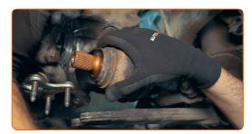
The outer CV joint is usually secured to the hub with a bolt or nut. You need to unstake the fastener or remove the cotter pin from it and unscrew it
