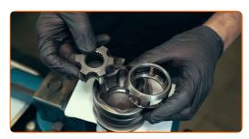
Remember the position of the inner race and where the circlip is located
