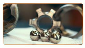
Check that the CV joint components are in good condition
