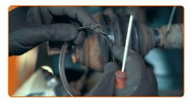
Detach the CV joint from the axle shaft
