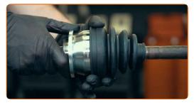
Install the clamps and make sure they are positioned correctly, without misalignment
