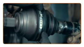
Removing this type of CV joint may require a special tool
