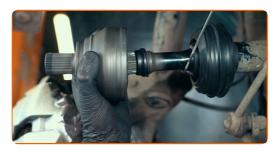
Push the CV joint to overcome the resistance of the circlip and click the joint into place
