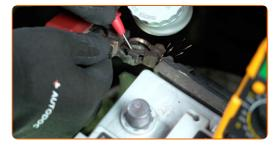
When installing a battery, you should, vice versa, connect the positive terminal first.
