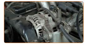
The positive one is connected to the car's electrical system containing the following consumers: a starter, ignition coils, electronic control units, various servos, headlights, an infotainment system, and other devices.
