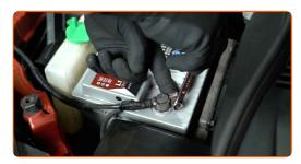
In the process of removing the battery terminals, you can accidentally touch its bracket, metal parts in the engine compartment, or the car body. In case you're removing the positive terminal first, this will lead to a short circuit.
