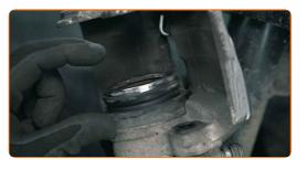
It should be wound back to its original position before installing the new brake pads. Use a special brake caliper piston wind-back tool
