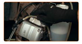
Clean any traces of brake fluid from the work area
