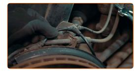
The last fastener should be the one located on the car body
