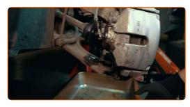
Follow the hose upwards, unscrewing all fasteners one by one
