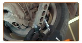
Take off the brake caliper and unscrew it from the hose, which stays in place.
