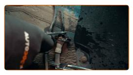
If the fastener starts to rotate together with the brake pipe, clean the nut and carefully loosen it
