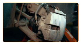
Alternatively, unscrew the brake line fitting and unscrew the hose from the brake caliper.
