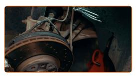
Unscrew the brake line fitting using a suitable tool
