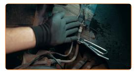
Remove the brake hose from its mounting seat by slightly twisting it.
