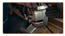
Make sure the system is leak-tight by pressing the brake pedal several times in a row
