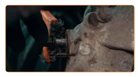
Install the brake hose. Use new sealing washers
