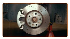
Treat the surface with an anti-corrosion agent
