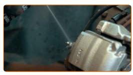
Bleed the system of air by pushing the brake fluid through it
