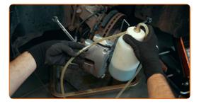
First, unscrew the bleeder screw slightly
