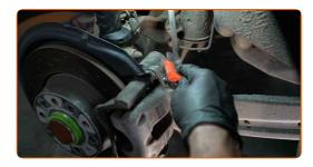
The assistant presses the brake pedal, which creates pressure in the system
