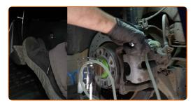
Brake fluid flows out of the bleeder screw and a new portion of it is supplied from the expansion tank
