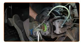
Tighten the bleeder screw and ask your assistant to release the brake pedal
