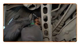
Perform the procedure on all calipers in order of decreasing distance from the expansion tank
