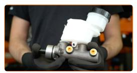
Start bleeding the system from the longest brake circuit which extends farthest from the tank
