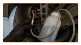
Check that there are no air bubbles and tighten the screw
