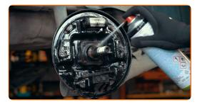
Treat all the surfaces and components with an anti-corrosion agent
