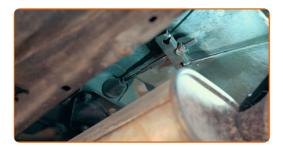
Loosen the handbrake cables using a suitable tool
