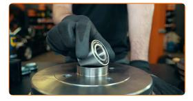
Lubricate the mounting seat and install the bearing
