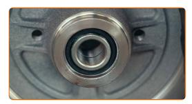
Fit in the retaining ring, which will help you determine if the bearing has been installed correctly
