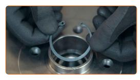
Install the ABS magnetic ring using a driver with a suitable diameter
