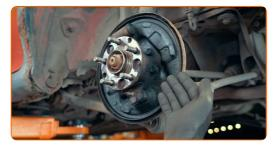
Before the replacement, compare the removed brake shoes with the new ones so that you don't install them on the wrong side. The brake shoes differ depending on the side of installation
