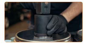
Adjust the position of the brake shoes before installing the brake drum on the stub axle
