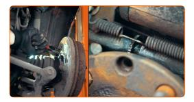
If the mechanism is corroded, use a slide hammer or special puller to remove the brake drum
