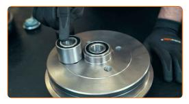
Position the driver and start hitting it with a hammer
