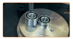
Pushing the inner ring can damage the bearing
