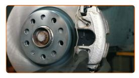
Treat the surface of the new brake disc where it will contact the wheel rim with an anti-corrosion agent
