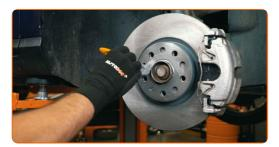
Clean the mating surface on the wheel rim and the working surface of the brake disc
