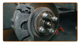
When doing this, you might need to remove the retaining spring, guide pin caps and guide pins themselves, and the fasteners of the brake caliper bracket
