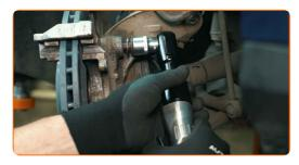
Check the condition of the brake hose and the brake caliper guide pins and piston boot
