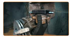
51 Install the brake caliper
