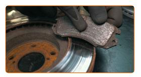
Discs can also be damaged from the inside due to corrosion
