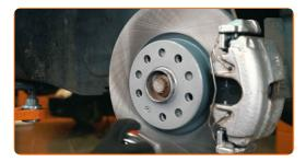
Screw in and tighten the wheel fasteners in a criss-cross pattern. This will ensure uniform fit of the wheel to the hub
