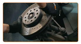
On many cars, the brake discs have an integrated wheel bearing
