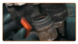
Wind back the brake caliper pistons. Use a special brake caliper piston wind-back tool
