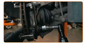
Clean and remove the fasteners that connect the brake disc to the wheel hub
