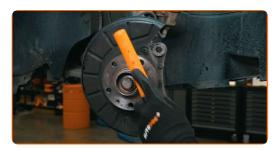
Treat the surface with an anti-corrosion agent
