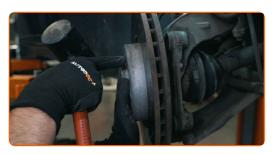
Hit it gently, just enough to create vibration without damaging the bearing
