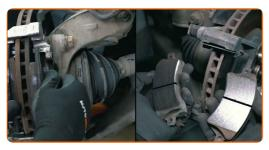
21 If the brake caliper has a bracket, remove it
