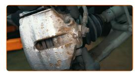
If the caliper is difficult to remove, use a suitable tool to force it apart or to pry it off
