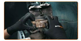
The caliper piston boot should not be damaged
