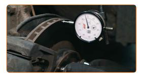
A corroded wheel hub prevents the disc from contacting the hub surface evenly
