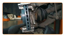
Tighten the fasteners with a torque wrench to the manufacturer's recommended torque
