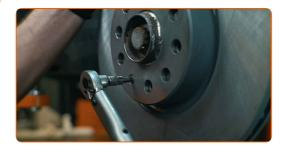
Clean the brake caliper bracket
