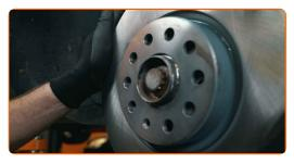
Install and tighten the fasteners with a torque wrench to the manufacturer's recommended torque
