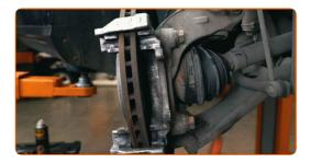
Clean and unscrew the bracket fasteners
