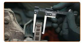
Worn discs may crack due to overheating
