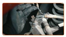
When replacing a caliper, it may be necessary to install a new bracket and guide pins if they are worn
