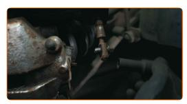
Unscrew and disconnect the brake caliper fasteners
