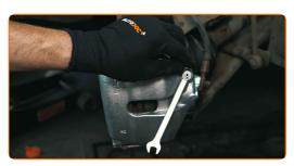
Repeat the procedure until all air is purged from the brake system
