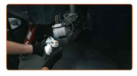
14 Disconnect the brake hose fitting
