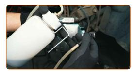
Connect this device to the bleeder screw on the caliper and loosen the screw slightly
