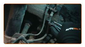
Fix the clamp on the hose at a right angle
