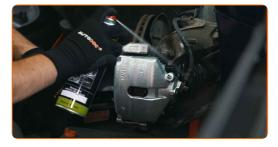
Tighten the bleeder screw to the torque recommended by the manufacturer
