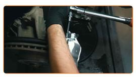
Install additional brake caliper retainers, if there are any
