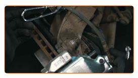
Remove the cap from the bleeder screw
