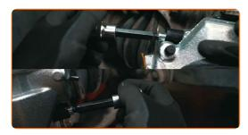
Tighten the fasteners to the torque recommended by the manufacturer
