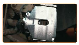
Corrosion may hinder the piston movement, and even cause it to seize up
