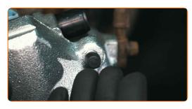
Undo the bleeder screw and remove the hose clamp
