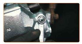
As soon as the fluid starts to leak out, tighten the bleeder screw
