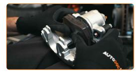
28 Install a new brake caliper
