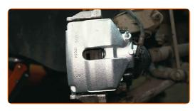
Put the protective cap on the bleeder screw
