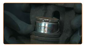
6 It can also be damaged as a result of destruction of the seal
