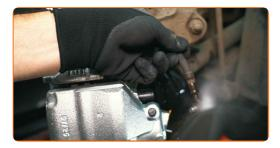
Tighten the fitting to the torque recommended by the manufacturer
